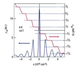
Measurement of Quantum Hall effect in graphene: the quantisation steps are easily detected: the quantised values are defined better than 1 part in 1 billion providing a new practical standard for resistence.
